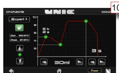
Possibility of adjusting the infusion curve after the cycle has been completed (on the BTA)
