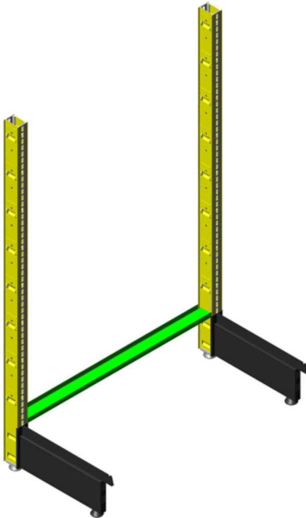
Hold two uprights the appropriate distance apart and insert bottom spanner into both uprights.
