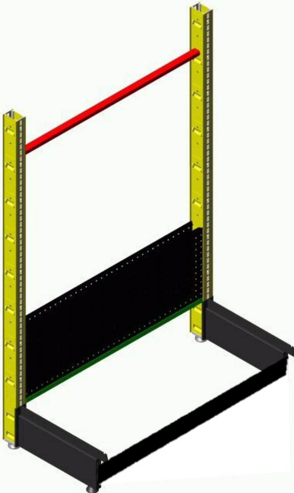
Attach kick plate to the base feet, then install the back panels into uprights.
