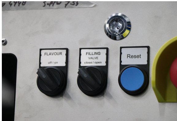
The center button operates the automatic valve
