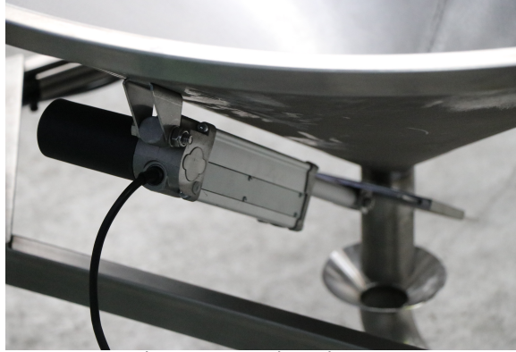
Linear motor that operates the valve
