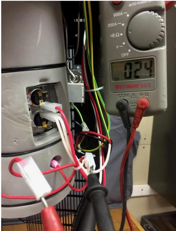
To replace heat band remove the black ties that secure insulation. Once removed pull heat band wires thru the insulation.
