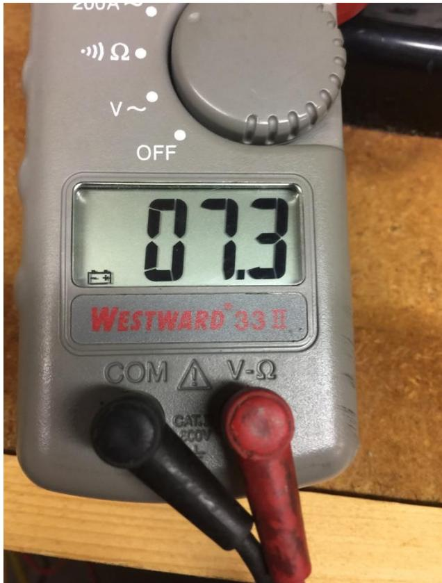
Reading should than settle down around 1 amp or slightly higher. If reading drops to zero for about 30 seconds than jumps back up to around 7 amps than down to zero. Replace both components.
