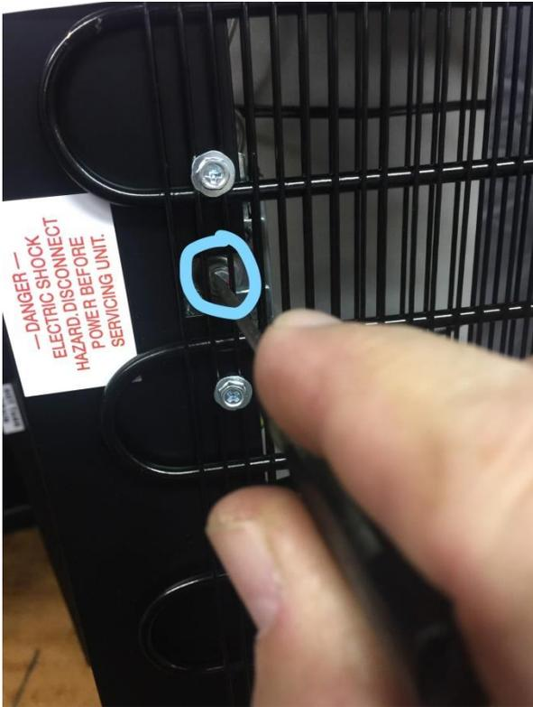
Check wires connected to cold control.
