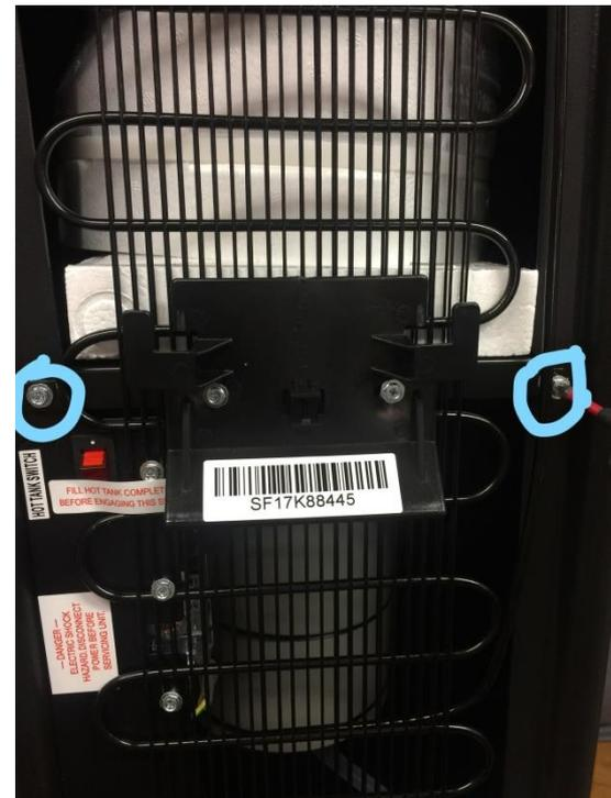
**Remove the 2 screws that secure cabinet to base pan.**
