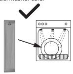
3. The filter must be DRY before you put it back into the holder.
