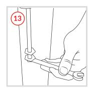
Secure the agitators to the spindle using a wrench.
