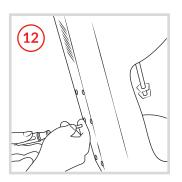
Secure the back cover using a screwdriver and the original six screws.
