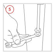
Remove the agitators from the spindle using a wrench
