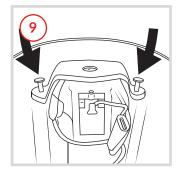
Secure the top plate using a screwdriver and the original two screws.
