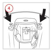
Use a screwdriver to remove the two screws from the top plate holding the motor in place
