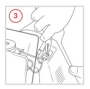
Remove the back cover by pulling it from the housing and unplugging the motor from the top of the cover.
