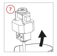
Lift the motor assembly straight up and out of the housing.
