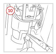
Plug the new motor into the housing just as it was before Step 6
