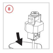
Lower the new motor assembly into the housing by guiding the spindle through the hole.
