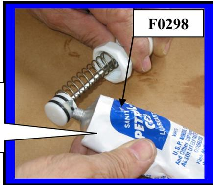
Installing **Plunger Assembly** into Faucet body
