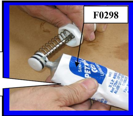
Installing **Plunger Assembly** into Faucet body
