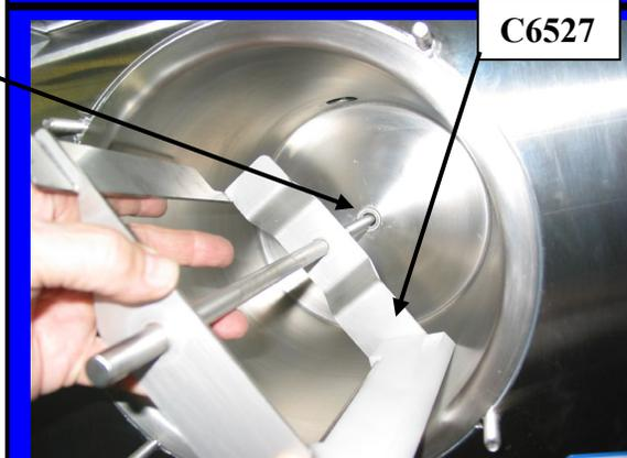
Carefully insert the beater bar C6527 (with beater seal) into the hole at the rear of the cylinder and rotate until it fully engages into the drive plate.
