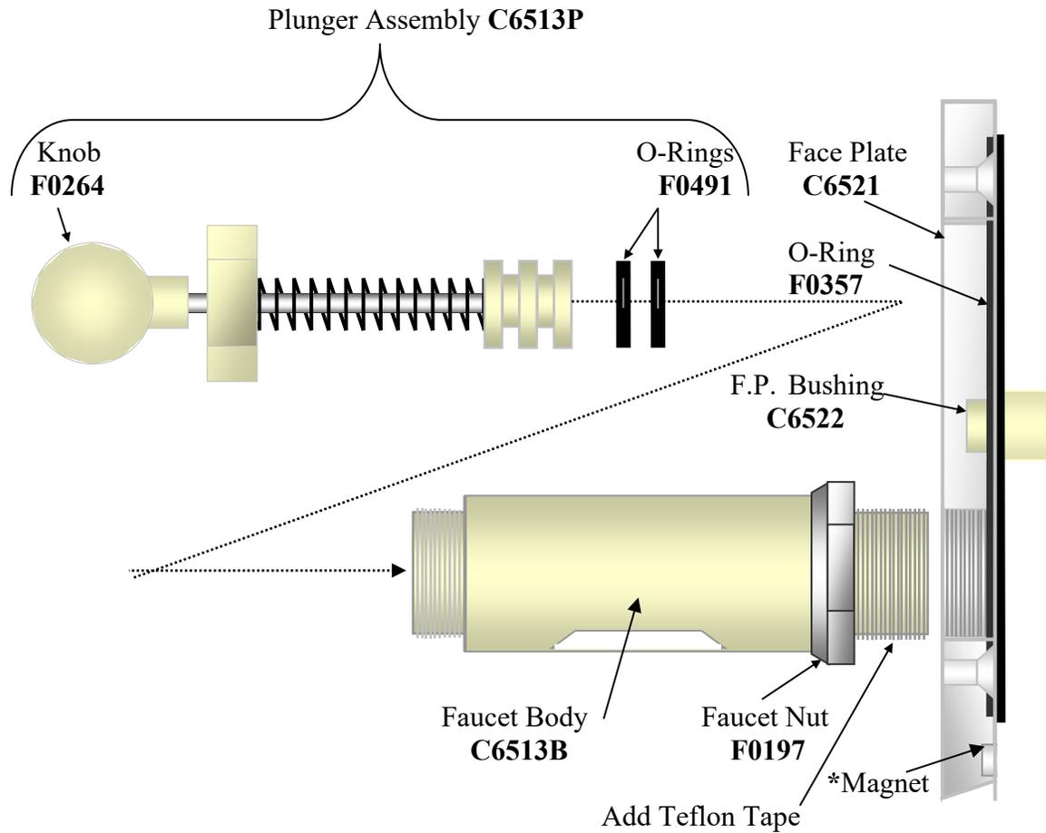
\*Motor Disconnect Magnet (Motor will not operate when faceplate is removed)
