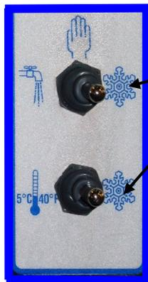
**Normal Operation** – Both switches on **snowflake**. Machine will freeze mix to provide frozen beverage as desired.
