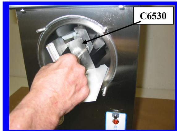
Re-install the **faceplate** on the machine. First place the faceplate **bushing** onto the beater shaft. Then slide face plate onto the four studs. Install the faceplate knobs and tighten evenly until the faceplate O-ring is snug against the cylinder.
