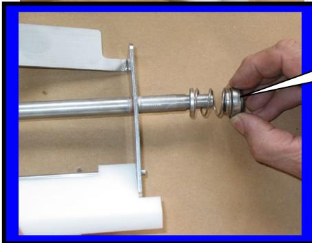
Step 5: Install spring seal F0355
