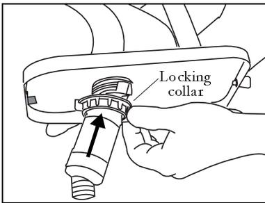
**2** Firmly insert long dip tube into bottom of pump.
