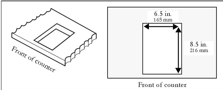
**2** With locking pin hole toward back of counter, lower dispenser container into hole until flange rests on counter top.
