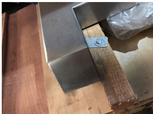
Figure 5. Bolts locking FRM-1120C to crate.
