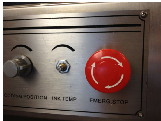
Figure 32. Remove Washer Holding Ink Temperature Potentiometer
