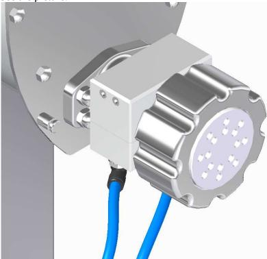
1-FRIO can be connected to the water supply with one tube-enter and one tube-exit. The cold water circulating in the system will cool the head during the extrusion.
