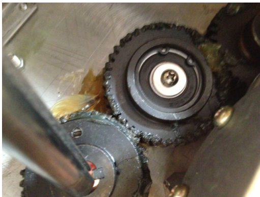
Figure 4. Ensure the groove in the long shaft matches that in the gear
