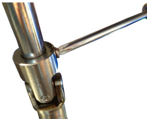
Figure 6. Screw the long shaft to the umbrella gear base.
