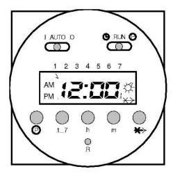
6. The skip cycle button, represented by an arrow with an X through it, probably will not be necessary in normal operation. If someone was going to be monitoring the pump on a daily basis and wanted to skip the next programmed function, the button would be depressed once and the symbol would show up in the lower right side of the display. The one situation where it might get used is outlined in Step #2 – 9 deleting a program setting (event).
