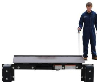
3. Pull the handle back until the leveler plate is vertical and the lip plate is fully extended.
