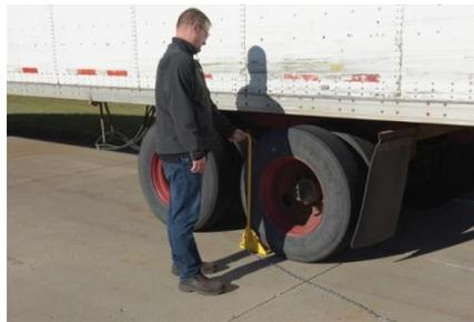
2. Remove the handle from the bumper box. Insert it into the socket on the left side of the leveler plate.
