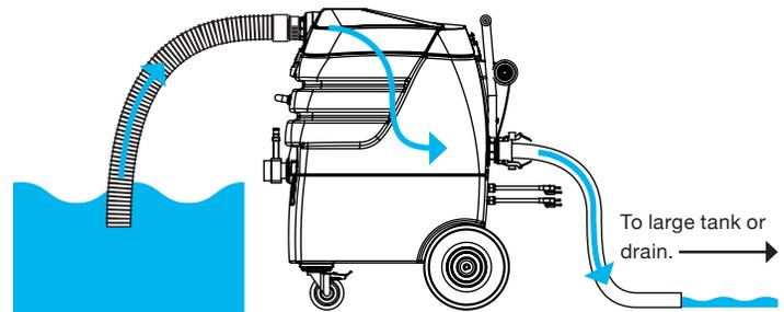
In shallow or light flooding situations, a flood wand can be used (included in the A138 Accessory Kit) for flood extraction. For heavier flooding situations, a stand-on flood extraction tool can be used or just a vacuum hose (included in the A138 Accessory Kit). ♦
