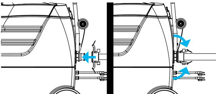
Attach the pump-out hose to the Auto Pump-out fitting. Secure the hose to the fitting using the cam lock. Push the hose cuff onto the fitting, making sure the silver ears and rings are extended forward. Pull the ears down using the rings until connection is tight. Place the end of the hose in
