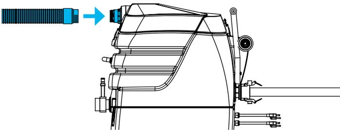
Vacuum hose can be connected to the Cuff-Lynx™ connection on the front of the lid on top of the machine. ♦
