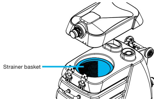
To keep the Flood Hog™ running smoothly for a long time, regular maintenance is necessary. Regularly inspect and clean the strainer basket, recovery tank, and all hoses. Also keep all wheels lubricated and check for leaks or loose hardware. ♦
