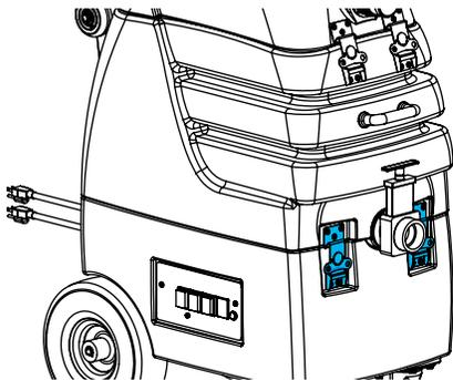
The Flood Hog™ can be opened for maintenance via the two lower latches on the front of the machine. ♦
