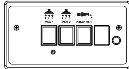
Switch on the vacuums using the two vacuum switches. Switch on the pump-out using the pump-out switch. ♦
