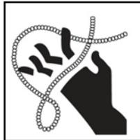
Do not overstress flexible shaft. Overstressing flexible shaft may cause twisting, kinking, or breaking of the flexible shaft and may result in serious injury.
