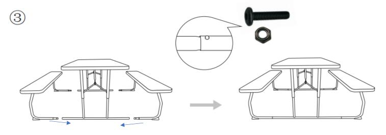
Insert the bottom of the legs of the seats into the legs of the table and attach using (4) 6x32 Bolts and (4) M6 Nuts.
