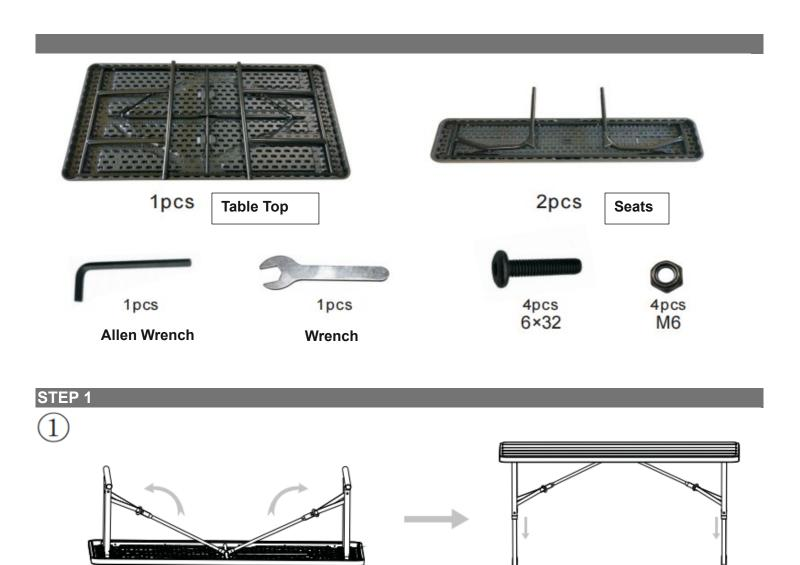
DIAGONAL BRACES MUST ALSWAYS BE IN THE LOCKED POSITION DURING USE.
