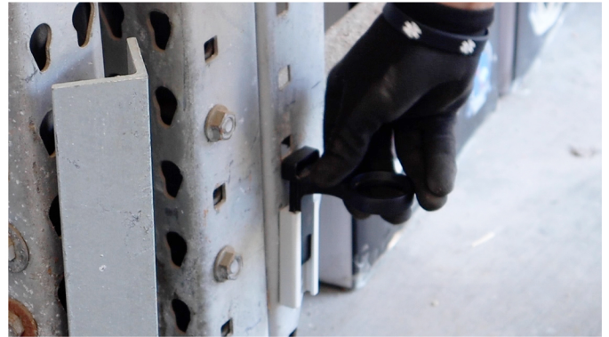
STEP 2. Slide the plastic bracket into the metal piece from the top. Make sure the plastic bracket is secure.
