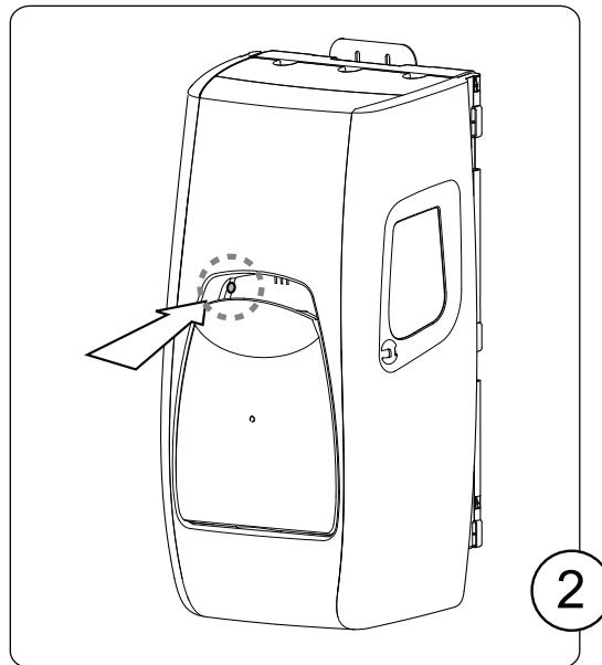
Push the blue button and hold for 3 seconds until a beep is heard to disarm the alarm.
