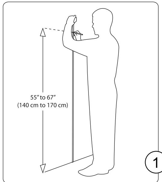
On a secure wall, using a tape measure (or the tape provided), mark anywhere between 55" and 67" (140 cm and 170 cm ).
