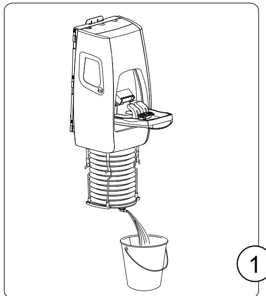
Following use and after injured person has sought medical attention, disarm the alarm by pressing and holding the blue button for 3 seconds until a beep is heard. Drain waste reservoir by placing an 8-gallon bucket under waste reservoir and open Drain Spout (turn to the right). If desired, a hose may be placed over the end of the drainspout to assist in emptying contents of waste reservoir.
