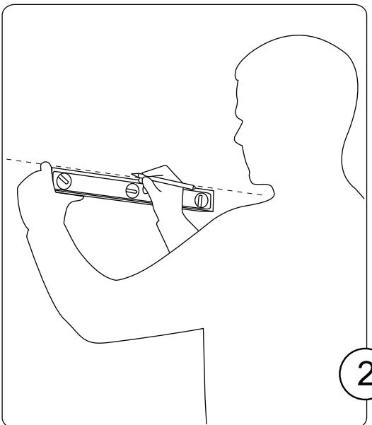
Use a level to draw a horizontal line at the mark made in Step 1.
