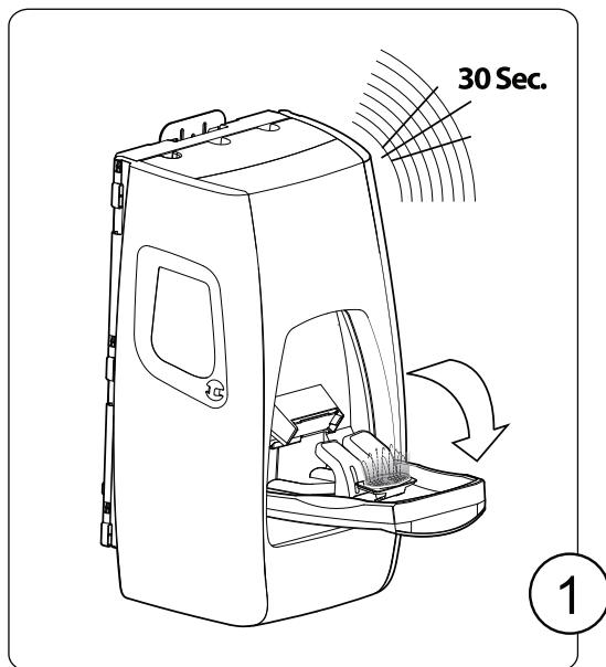
Pull on door to activate unit. Alarm will sound for 30 sec. to alert that the unit is activated.
