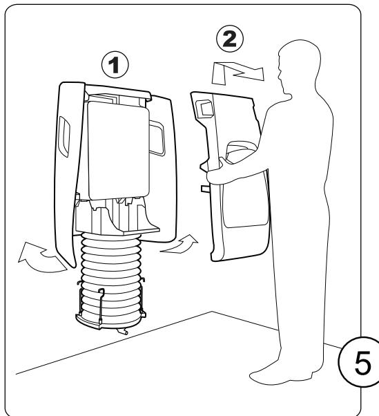
Open side panels by snapping them out of the front panel, remove the front panel by lifting upwards and then pulling forward.
