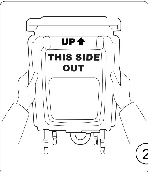
Hold cartridge using side handles, making sure the nozzle and tube are facing downward and the sticker on the front face of the cartridge is facing out.
