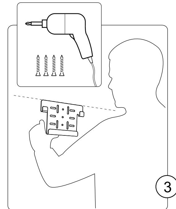
Align the top of the bracket with the horizontal line and mount the bracket. Mount with appropriate mounting hardware (not included)
