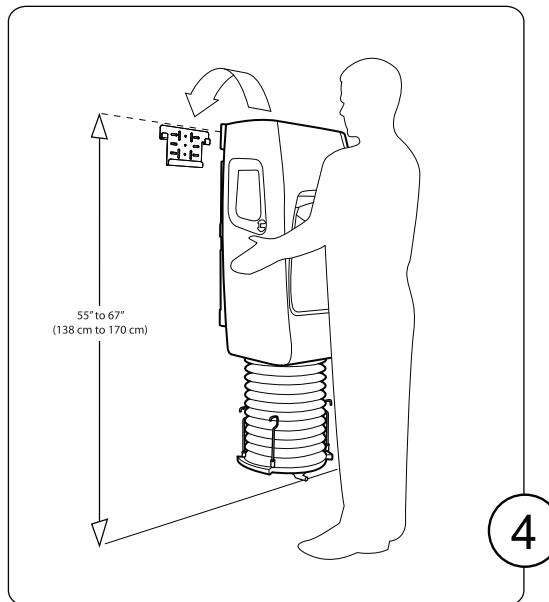
Keep unit assembled and hang it on the mounted wall bracket.
