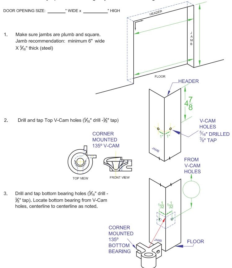
4. Remove adjusting nut and spring to install bottom bearing. Install the door leafs, bottom first.
