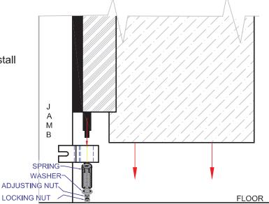
5. Shim if necessary - tighten bolts on V-Cam and bottom bearing. - tighten adjusting nut on spring compensator to achieve desired tension.
