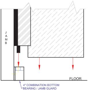
5. Shim if necessary - tighten bolts.
