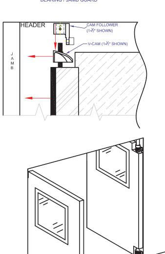
6. Make sure leafs swing freely in both directions. If doors do not swing freely, loosen bolts and re-align.
