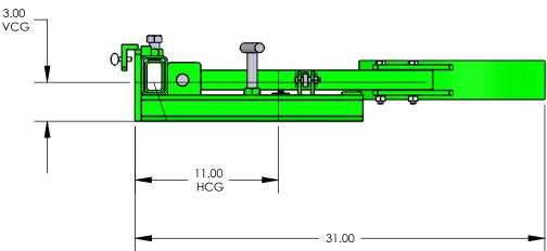
HCG = HORIZONTAL CENTER OF GRAVITY LC = LOAD CENTER LLC = LOST LOAD CENTER VCG = VERTICAL CENTER OF GRAVITY
