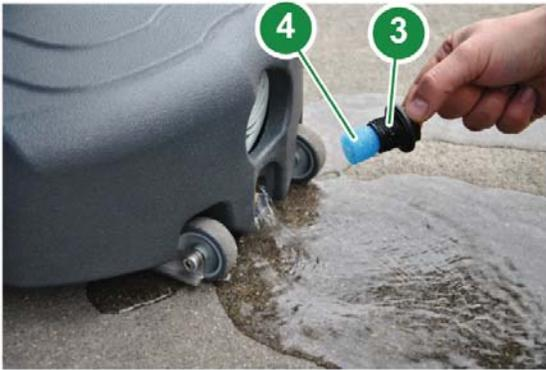
1. Unscrew the drain plug 3, together with the filter 4, located in the lower part of the tank.
