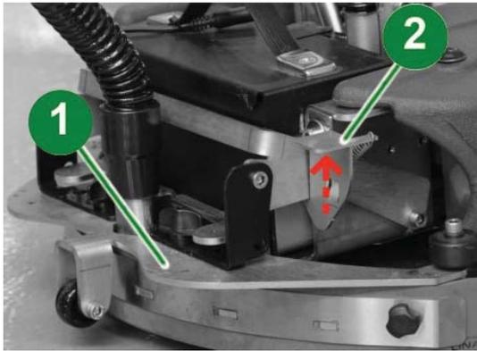
Lifting the squeegee off the floor from plate “1” activate the snap lock “2” which allows the squeegee to remain lifted from the floor.
