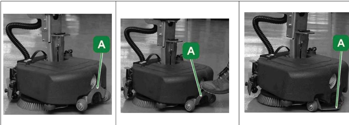
With the machine in POWER OFF, pressing and rotating the front lever A, the machine will rest on the three wheels and lifts the brushes OFF the floor. In this position it is possible to move the machine by maneuvering it as in the working phase without blocking the handle.
