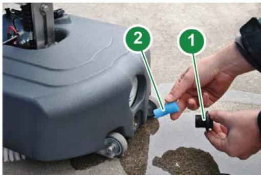
1. To clean the detergent solution filter, remove the plug 1 and the filter element 2.
