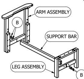
**2)** Attach (1) Support Bar to Arm Assembly and Leg Assembly using (4) "B" Bolts as shown.
