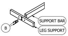
1) Attach (1) Support Bar to Leg Support using
