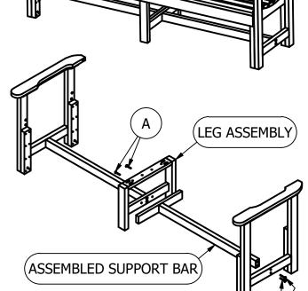
**3)** Attach the Assembled Support Bar to the Arm Assembly and Leg Assembly using (2) "A" Bolts and (2) "B" Bolts as shown.
