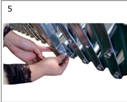
6. Fasten cross bar to each leg with M10x16 bolt.
