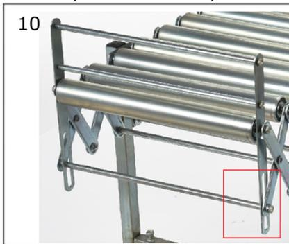
**Remove bolt & washers on both sides of rod. Insert rod through slots in stopper bracket. Reinstall bolts and washers. Tighten bolts.**
