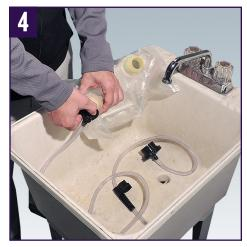
Attach the hose assembly to the cleaned out bag (if you did not clean the bag used for finishing/mopping, you can attach an empty replacement bag to continue the hose assembly cleaning process: Part No.: EFBAR).
