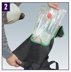
If cleaning the fluid bag, remove it from the backpack, properly discard any remaining finishing/cleaning fluid per manufacturer instructions and rinse out the bag with clean warm water.
