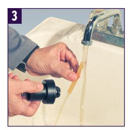
Rinse the valve assembly and dispensing tube with clean warm water. If the dispensing tube at the base of the valve assembly is clogged, flex the tube slightly to loosen the clog. If this does not work, replace the tube (Part No.: EFTDS).
