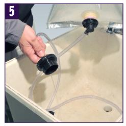
Run clean warm water through the bag and hose assembly to rinse the finishing/cleaning fluid from the hose.
