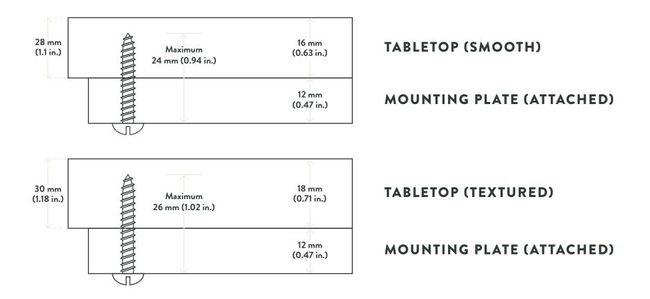
A minimum screw length of 1/2" should be used, but a screw length of 3/4" is recommended for installation.
