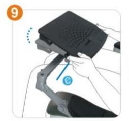
Press button and rotate the support board for adjusting the best position according to different tilt sitting posture.
