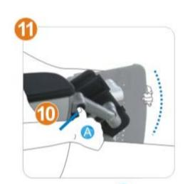
Press button (A) and rotate the support board backwards by 90° with left hand, then the support stand is locked automatically with a "click" sound.
