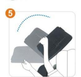
Use your right hand hold buttom (B) and turn the support board rightwards with 135°.
