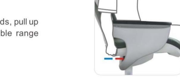
Push the backwards tilting handle with right hand to Unlock position, unlock the backrest tilting when hear the "click" sound; Then recline to the desired position,
