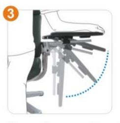
Turn up the support board by rotating it upwards to 90°.
