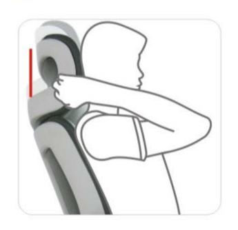
Hold the frame of headrest with both hands, pull up or down to adjust the height. The adjustable range would be 100mm.
