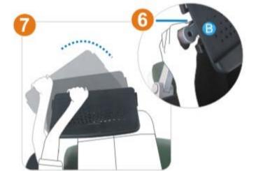
Re-press the locking buttom (B) to adjust the support pole in a suitable angle, it could be adjusted with 45° range and there are three positions locking.
