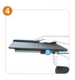
Open the support pole locking system by pushing the buttom (B) as the direction of the arrow.
