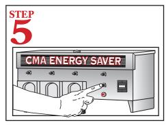
Press the "FILL/START" switch. Hold in the "FILL" position until the water overflows into the scrap accumulator.
