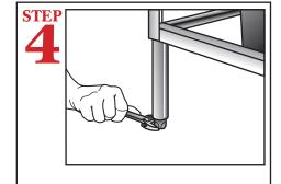
Level dishmachine by adjusting leveling legs. Dishmachine must be level front and back to ensure proper performance.
