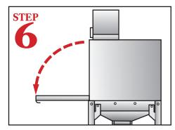
Open dishmachine doors completely. Closing the door will automatically activate the machine.
