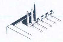
Lay paper horizontally (or flat), then return handle to vertical position to close comb.
