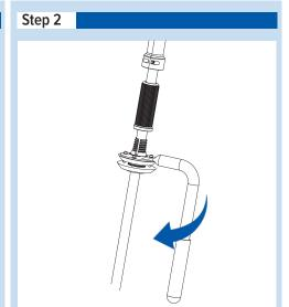
2. Loosen the Handle, from the Tube Adaptor by unscrewing it.
