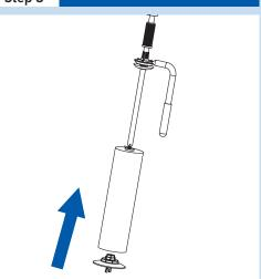
3. Slide the stretch film roll onto the Conduit Tube.
