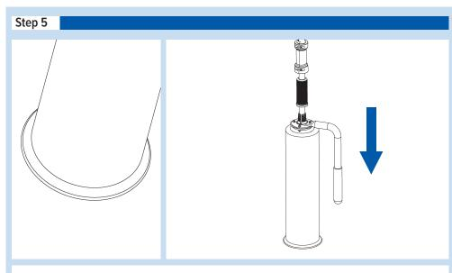
5. Once those parts are in place, position the stretch film roll so it is concentric with the Bottom Disk (1). Push the Handle down until the bottom disk of the handle is up against the stretch film roll. Hold the core of the Handle down with force, as you screw the Tube Adaptor into the Handle.
