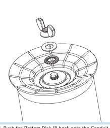
4. Push the Bottom Disk (1) back onto the Conduit Tube. Proceed to add the Flat Washer, Thrust Bearing, and Flat Washer. Screw in the Wing nut only until a third of the rod is in.
