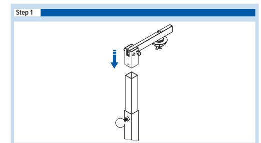
1) Slide Arm Support Assembly onto the Mast so that the top of the Mast is flush with the cut out of the Arm Support Assembly.
