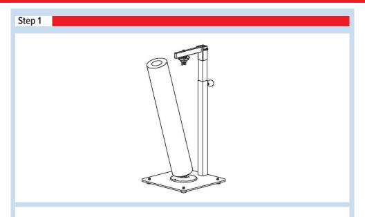
1) Grab and align the lower end of the roll with the bottom core of the dispenser.
