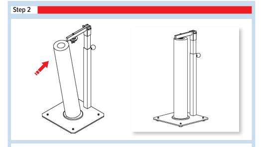
2) Next, use the telescoping height to adjust the top arm so that it is snug above the roll, with the core in the center of the roll.
