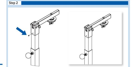
2) Then secure Arm Support Assembly to the mast with the Plug Screw.
