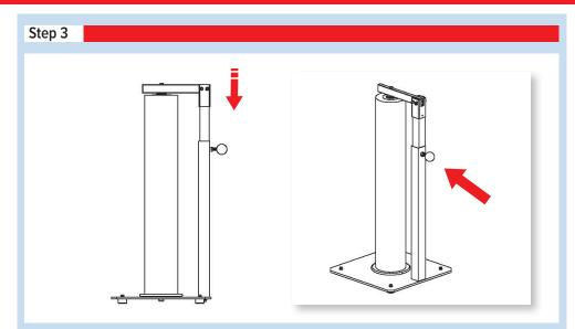
3) Once the roll is in place, apply downward pressure to the top arm as you secure the mast in place with the knob located on the side of the vertical frame.
