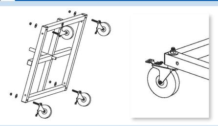
1) Flip the base frame onto its side and slide 5" casters (four) into their designated holes. Using a 3/4" wrench, screw on nylock hex nuts (four) and flat washers into the base frame (four).
