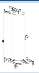
**Note:** Cutter blade cuts paper by sliding down attached cutter rail on the side of the back frame. Corrugated roll can be fed through the gap between the back frame and around the cutter rail.
