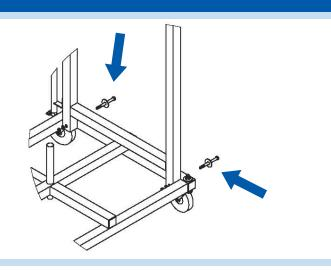
2) Once the base frame is standing, lock the 5" casters in place. Wiggle the back frame into the base frame and attach using 9/16" wrench (two), hex head bolts (two), flat washers (two outside back frame), and washers (two inside back frame). Use synchronized twists on both sides in opposite directions.
