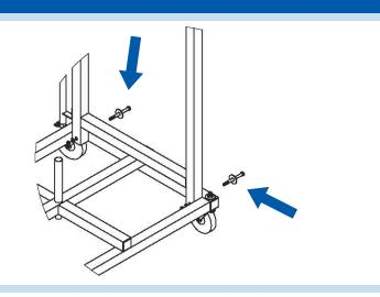
2) Once the base frame is standing, lock the 5" casters in place. Wiggle the back frame into the base frame and attach using 9/16" wrench (two), hex head bolts (two), flat washers (two outside back frame), and washers (two inside back frame). Use synchronized twists on both sides in opposite directions.
