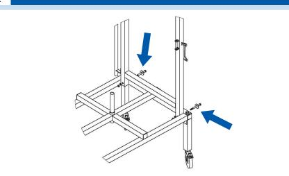
2) Once the base frame is standing, lock the 5" casters in place. Wiggle the back frame into the base frame and attach using 9/16" wrench (two), hex head bolts (two), flat washers (two outside back frame), and washers (two inside back frame). Use synchronized twists on both sides in opposite directions.
