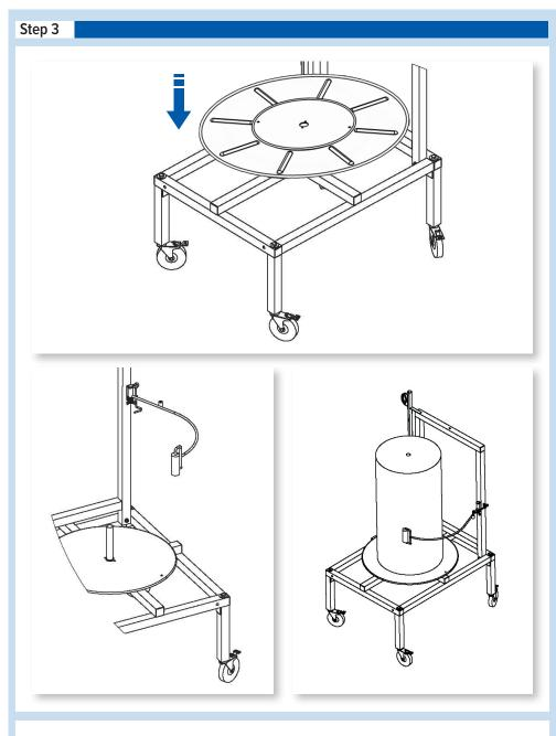
3) Next, slide the dispensing disk over the central cylinder in the middle of the base frame. At this point, the brake arm can be adjusted to size and a corrugated roll can be placed on top of the dispensing disk.
