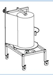
**Note:** Cutter blade cuts paper by sliding down attached cutter rail on the side of the back frame. Corrugated roll can be fed through the gap between the back frame and around the cutter rail.
