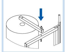
4) To attach the top arm, place on top of back frame and screw in a hex head bolt with flat washer on top and a washer with a nylock hex nut underneath, using a 9/16" wrench.
