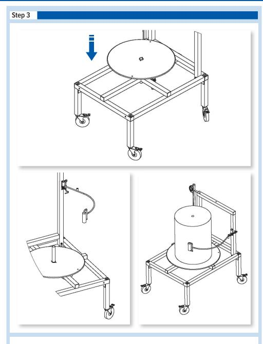
3) Next, slide the dispensing disk over the central cylinder in the middle of the base frame. At this point, the brake arm can be adjusted to size and a corrugated roll can be placed on top of the dispensing disk.
