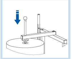
5) Once the top arm is firmly connected, hold bottom core (top) and "o" ring (bottom) in between the corrugated roll and against top arm. Slide adjuster through the designated hole in the top arm and through the core, "o" ring, and corrugated roll.
