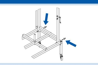
2) Once the base frame is standing, lock the 5" casters in place. Wiggle the back frame into the base frame and attach using 9/16" wrench (two), hex head bolts (two), flat washers (two outside back frame), and washers (two inside back frame). Use synchronized twists on both sides in opposite directions.
