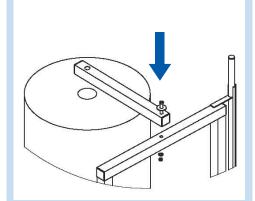
4) To attach the top arm, place on top of back frame and screw in a hex head bolt with flat washer on top and a washer with a nylock hex nut underneath, using a 9/16" wrench.
