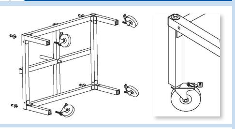
1) Flip the base frame onto its side and slide 5" casters (four) into their designated holes. Using a 3/4" wrench, screw on nylock hex nuts (four) and flat washers into the base frame (four).
