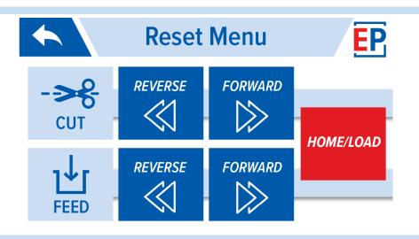
In this screen, press the button that reads "HOME / LOAD" and this will move the cutting mechanism to the correct position. Next, press the back arrow on the top left of the screen to go back to the main menu.
