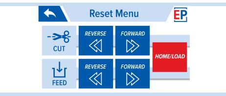
Next, the machine needs to be unjammed. If the material got stuck in the feed rollers, use the reverse button and forward button next to the feed symbol to move the material back out.
