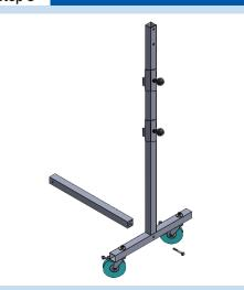
3. Attached the base couplers, perpendicular, onto the inside of both support stands.
