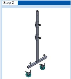
2. Use the provided washers and nuts to attach the casters on both sides of the support stand.
