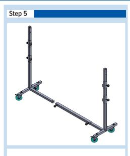
5. On one side, slide the base tube over the base coupler and tighten by twisting the ball knob.
