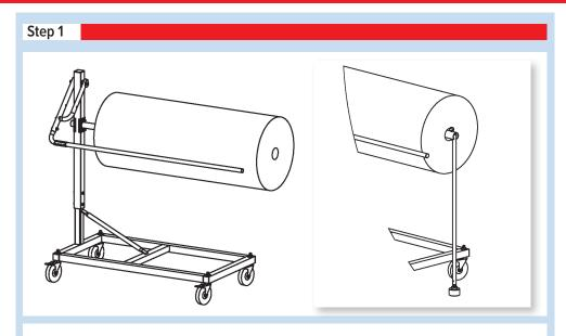
1. Load a roll onto the roll arm (E6450-07-A), and then pull out the support assembly (E6420-03) from within the roll arm and set it with the foam stopper against the floor.
