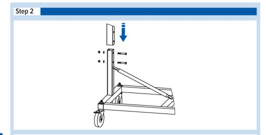
2. Attach the upper mast (E6450-01-C) to the base assembly (E6450-01) by sliding it over the lower mast. Check that the end with the two holes is facing downwards. Fasten together with two hex bolts (E6420-12), two washers (E5960-04), and two nylock nuts (E3065-19).
