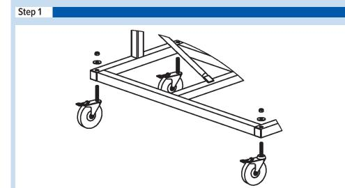
1. Insert casters into each hexagonal cut-out on the corners of the base assembly. Secure with four washers (E800-06-D) and four hex nuts (E6420-03-G). Engage caster brakes by pressing down the lever on the top of the casters.
