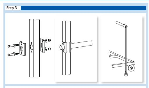
3. Check that the curved edge of the clips is facing each other and that the notch in the mount arm is facing down. Then slide the roll arm assembly into the upper mast until it passes through 1". Tighten nuts and bolts to secure roll arm assembly.
