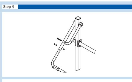
4. Insert the short end of the brake arm (E6450-08) into the extension arm (E6450-25-A). Check that the brake arm is in the same direction as the roll arm assembly. Secure in place by using the acorn nut (E5920-11), and two hex bolts (E6250-18), the longer bolt tightened above the shorter bolt.
