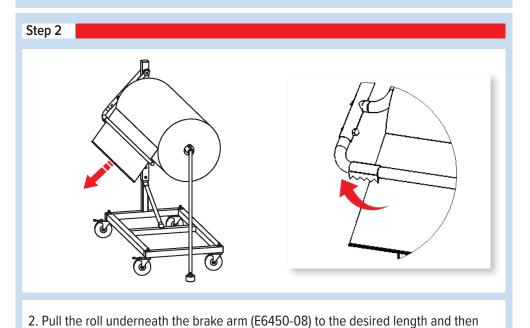
use the tear tag assembly (E6220-08) to tear off the piece from the roll.
