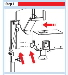
1. Carefully, hold up the feedbox and align it to the two bracket holes with the holes on the tube on the upper frame.
