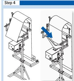
4. Once it's over the pvc tube, hand crumple the paper end, so it can be stuck through the crumpler attachment, and then slide into the crumpler chute.
