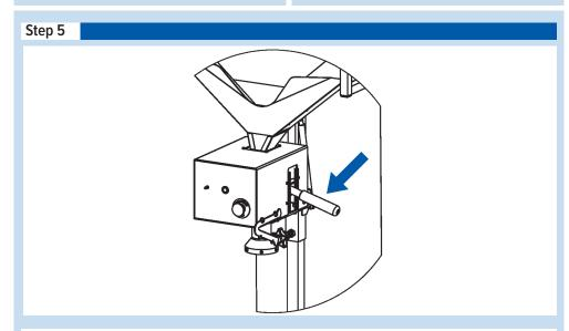
5. Engage the rollers by pulling down on the side handle, allowing the paper to be engaged with the rollers.
