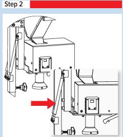
2. With caution, hold the feed box up against the holes and screw in the 2. ½-13" x 2 ½" bolts that are included. Secure tightly.
