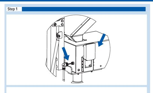
1. To begin loading and usage, plug in battery and foot pedal to the feed box.
