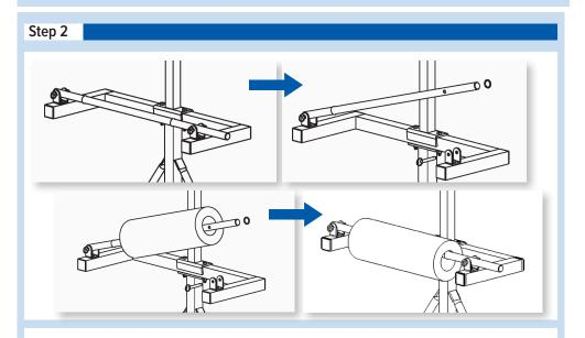
2. On the back bar, remove the quick release pin, and slide the o-ring off.
