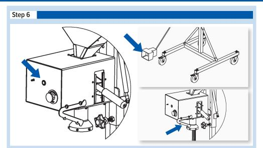
6. Push and hold the front button on the feedbox, or step on the foot pedal to dispense the paper. When the paper is at the desired length, cut using the blade on the side of the crumplers by pulling the paper against it.
