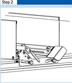
2. Align channel with a 3/8" locknut and slot on the back plate (#2). Use a 3/8" screw to secure the dispenser to the shelf using the shelf channel.
