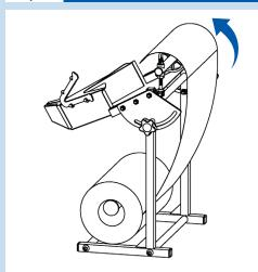
3. Pull paper upward and over the PVC roller.
