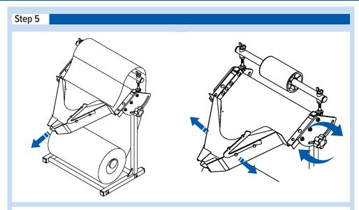
5. Feed the paper through the chute and use the cutter to cut paper to desired length. Adjust the positioning of the dispenser as needed by unscrewing the pivot plate knob enough to swing the chute into the position needed then secure in place by screwing in the knob.
