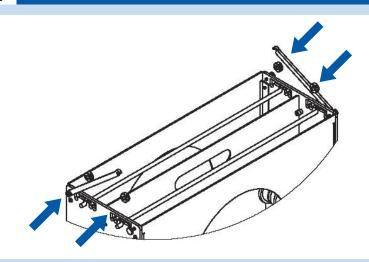
2) Loosen shaft collars on both sides of the polyurethane flanges, using a 9/64 Allen wrench/key. Slide polyurethane flanges to the size coil roll width and hold in place by re-tightening the shaft collars on either side.
