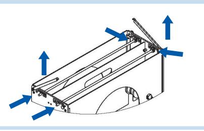
1) Lift bar lock to release retaining rod and move rods into designated notches, depending on the width of the coil roil. Once rods are adjusted, lock them in place by lowering bar lock.
