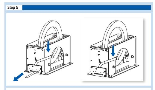
5) From outside of the dispenser, pull coil to desired length, and cut by pushing down on the cutter's handle.
