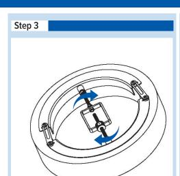
3) After being fully extended, rotate the adjustment handle until the tension is secure.
