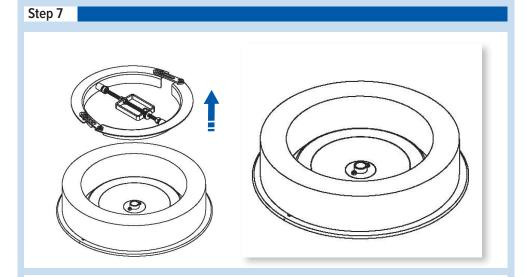
7) Finally, pull the EP-3003 out of the core of the roll as the roll now sits secured on the disk.
