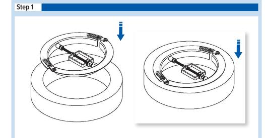
1) Place the EP-3003 within the diameter of the roll so that the forming arms are against the side of the roll.
