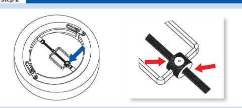
2) Once the forming arms are flat against the roll, press the quick release to extend the forming arm as far as possible to maximize the tension holding the roll.
