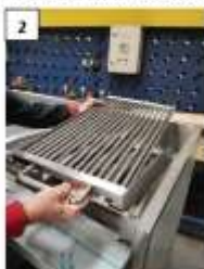
2 TOP GRILLS REMOVED
