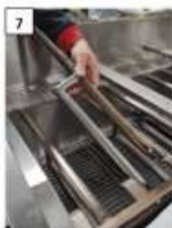
7 THE BURNER IS REMOVED
