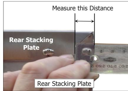
8. Place Front Stacking Plate on front top edge of Proofer and mark measurement taken at Item 7, to ensure Front and Rear Stacking Plates are aligned correctly.
