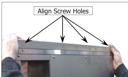
5. Align screw holes in Rear Stacking Plate with screw holes in rear of Proofer and secure in place with 4 screws.
