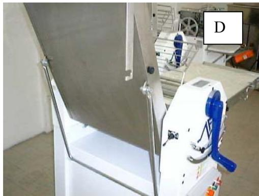
4. Remove the “spring pin” of the handle [picture E, F] and then the handle.
