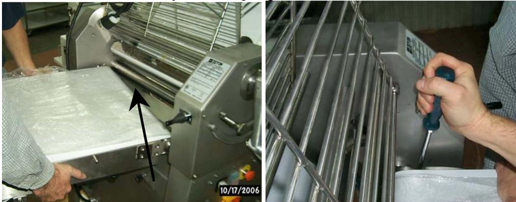
In same time you push the spring load, insert the opposite side of the conveyor in the front slot.
