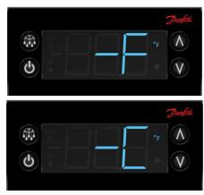
7. Push the defrost button (upper left button) to move out of the display unit menu.
