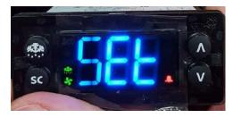
8. Adjust to desired setpoint and press lower left button to enter the new value into the controller.
