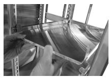
7. Install a bin in between each pair of C channels, pushing up the bin top as you slide the bin in.
