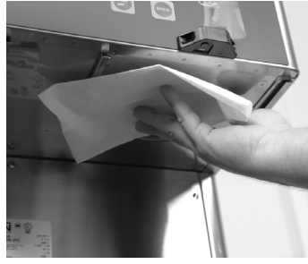
2. Use a clean damp cloth rinsed in mild, non-abrasive detergent to clean both sides of the sprayhead panel.
