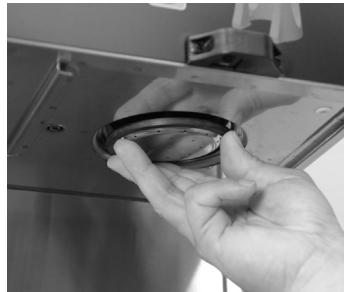
6. Reassemble sprayheads and reattach. Sprayheads only need to be hand tightened.
