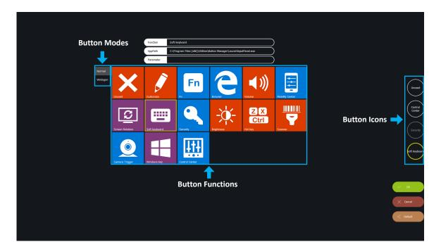
The Button Icons are located close to physical button locations. The icons show current assigned function. Button functions section will list all available functions for current system model.
